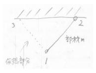
$$\{F\}_{m} = \begin{cases} X_{1} \\ Y_{1} \\ X_{2} \\ Y_{2} \end{cases} = \frac{A_{m}E_{m}}{2l_{m}} \begin{bmatrix} 1 & 1 & -1 & -1 & 0 & 0 \\ 1 & 1 & -1 & -1 & 0 & 0 \\ -1 & -1 & 1 & 1 & 0 & 0 \\ -1 & -1 & 1 & 1 & 0 & 0 \end{bmatrix} \begin{pmatrix} u_{1} \\ v_{1} \\ u_{2} \\ v_{2} \\ u_{3} \\ v_{3} \end{pmatrix} \cdots 2 -1$$
