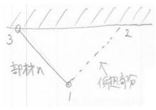
$$\{F\}_{n} = \begin{cases} X_{1} \\ Y_{1} \\ X_{3} \\ Y_{3} \end{cases} = \frac{A_{n}E_{n}}{2l_{n}} \begin{bmatrix} 1 & -1 & 0 & 0 & -1 & 1 \\ -1 & 1 & 0 & 0 & 1 & -1 \\ -1 & 1 & 0 & 0 & 1 & -1 \\ 1 & -1 & 0 & 0 & -1 & 1 \end{bmatrix} \begin{bmatrix} u_{1} \\ v_{1} \\ u_{2} \\ v_{2} \\ u_{3} \\ v_{3} \end{bmatrix} \cdots 2-2$$
