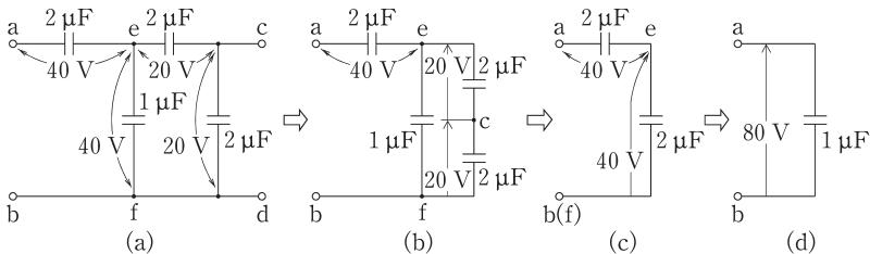
$$\text{図(b)} : C_{ef} = 1 + \frac{2 \times 2}{2 + 2} = 1 + 1 = 2 \mu\text{F}$$
