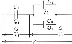
$$Q_2 = C_2 V_2 = 4 \times 10^{-6} \times 80 = 320 \times 10^{-6} \text{ C} = 320 \mu\text{C}$$
