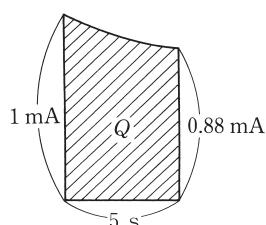
$$(2) \quad v_C = \frac{Q}{C} = \frac{4.7 \times 10^{-3}}{400 \times 10^{-6}} = 11.8 \text{ V}$$
